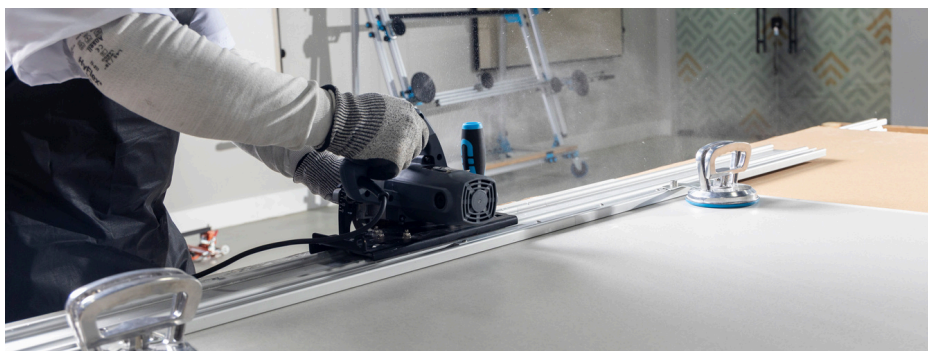
Image 77: Slide the marble saw along the rail, without forcing the disc to advance across the piece.
