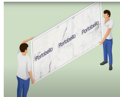
Image 06: Correct handling of slabs.
